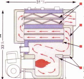
**EFM'S EXCLUSIVE** *Turbo-Ram* **DESIGN TURBULATORS** force more heat against boiler tube walls for unsurpassed heat-transfer efficiency.
